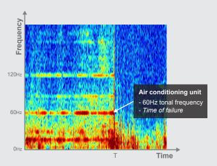
Failure of the air conditioning unit in a telecoms room at a remote block valve station had led to the shut down of critical electronic equipment due to over heating, resulting in pipeline shut down.
